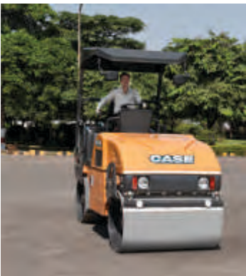
High kerb clearance for effective operation alongside culverts.
