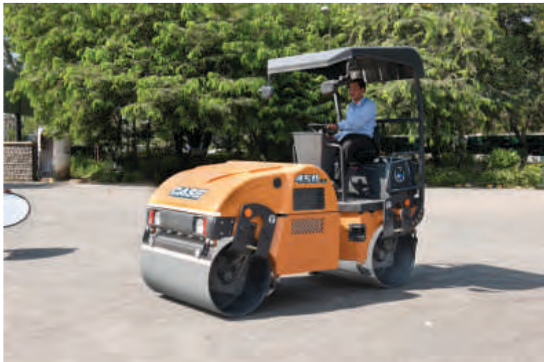
Compact design - equal distribution of weight for even compaction. Even distribution of load during transportation.
