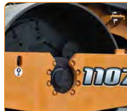
Heavy Duty Frame with 32mm Drum Shell
